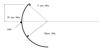
12.5. Recesses in the hull or deck for the purpose of hiding bolt or screw heads etc. are to be permitted. Recesses should be safer than a projecting fixing device in order to be legal. Where recesses are provided to improve safety by eliminating projecting fixing devices, the 5mm radius shall be relaxed as far as it would cover the radius of any transition curve between the deck and the side surfaces of any such recess.
