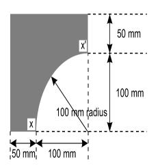
**4.3.** Gauge 3, depth gauge, 160 mm rise, must be used to measure section CC' to DD' (cockpit area).
