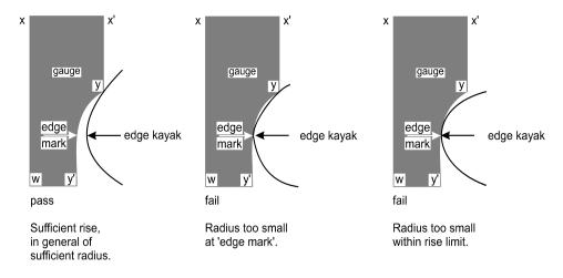
**3**. To gauge the radius of curvature the radius portion of the appropriate gauge, must be applied perpendicular to the surface being tested. If both points X and X' touch the surface at the same time without the rest of the kayak, the test is passed.
